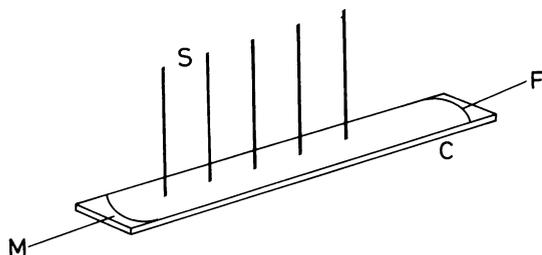
Fig. 1 Diagrammatic drawing of the recording set up. Segment of colon ( $5 \times 30$  mm circular muscle cells facing up with their long axis parallel to the long axis of the muscle segment) is indicated by a C. M = micromanipulator to adjust stretch. F = force transducer to record tension. S = suction electrodes to record electrical activity, placed 5 mm apart. One reference electrode was placed in the organ bath solution (not shown).
