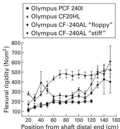
Figure 1 Mean (SD) flexural rigidity measurements ( $N\text{ cm}^2$ ) of three different colonoscopes: (a) Olympus PCF 240I, (b) Olympus CF20HL, and (c) Olympus variable stiffness CF-240AL instrument in its "floppy" and "stiff" modes.
