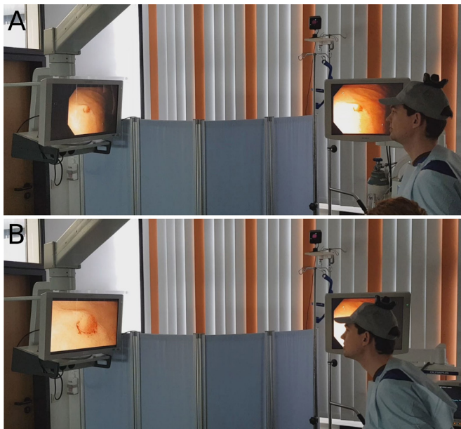
Figure 3 Intuitive zoom applied during gastroscopy. (A) Depicts the room setup with the monitor on left side and the examiner with the tracking device on his head on the right side. (B) Forward movement of the head results in a stepless magnification of the endoscopic image in the area of interest.
