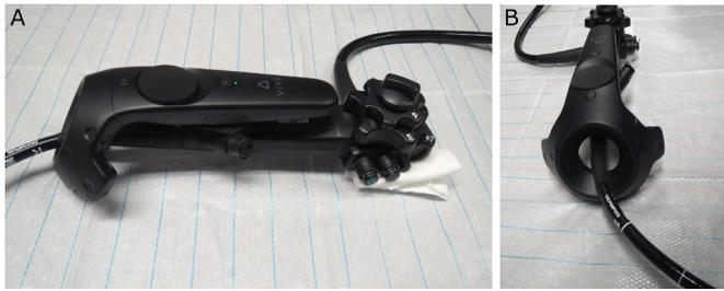
**Figure 1** Virtual reality-controller mounted on a regular gastroscope.
