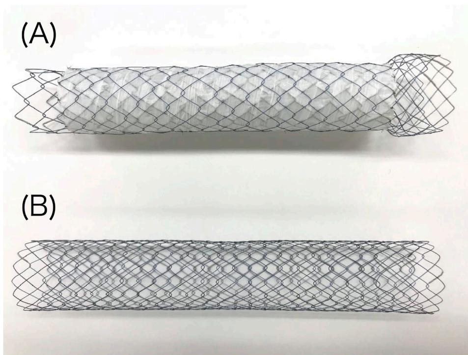
**Figure 1** Covered and uncovered self-expandable metallic stent (SEMS) used in this study. (A) The covered SEMS has an antimigration system at both ends (proximal uncovered flare and distal uncovered area). (B) The uncovered SEMS is straight and contains no membrane.
